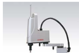
Hollow shaft option for easy routing of air tubes and harness wires
