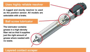
The dual-layer scraper prevents micro-contaminants adhering to the rod from penetrating to the inside. This is also effective in suppressing looseness or vibration in the rod.
