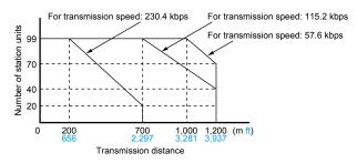
When using a transmission speed of 38.4 kbits/sec. or less, you can set up a maximum of 1,200 m 3,937 ft and 99 units. For RS422 setting, you can set up a maximum transmission distance of 400 m 1,312 ft.
