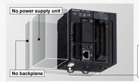
A 24 V DC power can be directly connected from the control panel.
