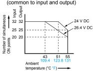
Note: Reduce load current according to the graph below by the external power supply voltage.
