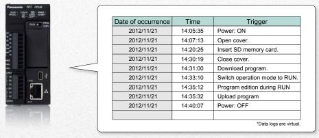
Operational events to CPU and program editing events are logged. Automatic logs of program download and upload are useful, especially for program debugging.
